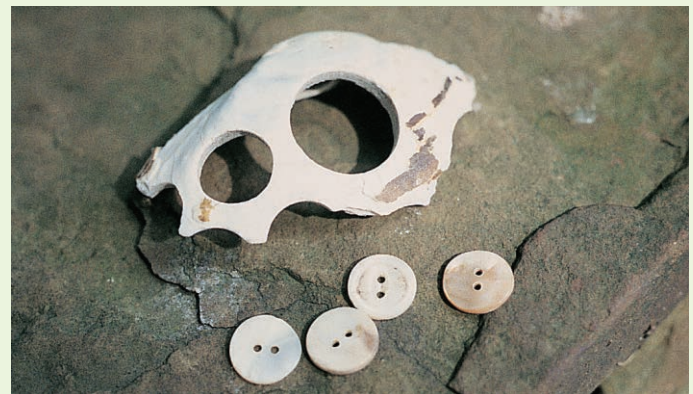
BOX FIGURE 11.3 Shell of a Freshwater Mussel after Having Been Drilled to Make Pearl Buttons.
